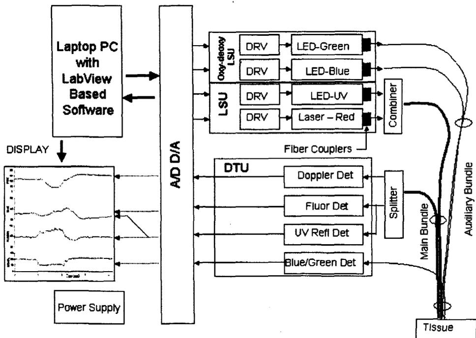
Fig. 4. Blocks Diagram of the TiSpec03 (for details see text).
